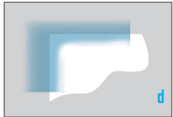
6: Let the MagneCoat dry for at least 45 minutes. Then apply a second layer of MagneCoat on top of the first layer. Let this layer also dry for at least 45 minutes. Afterwards, clean all of the paint out of the roller pan.
