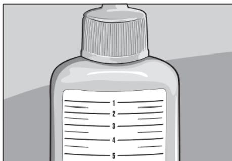
3: Open the bottle and pour the correct amount of ContrastBooster into the large container of BaseCoat. Stop now and then and set the bottle on a flat surface to check the amount that still remains to be added. Slowly add the last amount of ContrastBooster until the level in the bottle reaches the calculated number.
