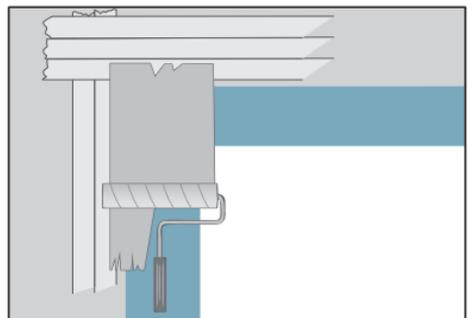
Special note!!! Apply the layer of BaseCoat on the inside and about 15 cm away from the tape on top of the magnetic paint (see illustration).
