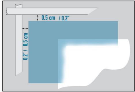
Make the adhesive band wider by applying a second strip next to the first strip. If you have enough tape, stick a third strip above the others. If you still have tape, stick a third strip on the bottom as well. (see illustration).
