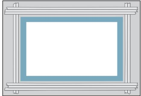
Check: Turn the projector on. The distance between the illuminated image and the tape must be exactly 5 cm / 2" (if you have the MPW 20 product) or exactly 7 cm / 2.8" (if you have the MPW 30 product). (see illustration). Turn the projector off again.
