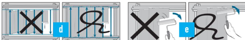
You should only change the direction of painting on the tape border. That means not on the screen! (see illustration d).
