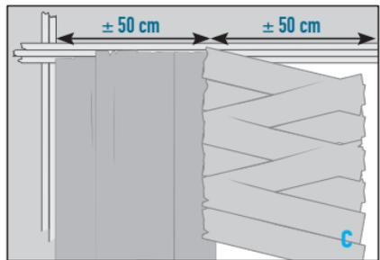
Let this layer dry for at least 60 minutes. During drying, place the roller in the roller pan and make sure that it is covered with sufficient paint to prevent it from drying out.
