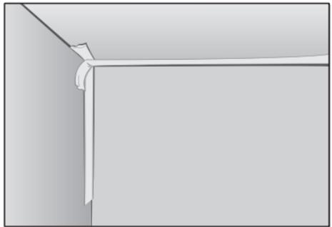
b. In instruction 3, you paint just one band of BaseCoat, about 15 cm wide, on top of the band of MagneCoat (see illustration).
