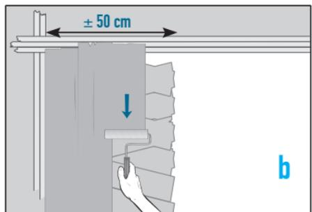
Always apply the paint fully "wet on wet".
